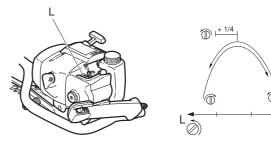
**CAUTION!** If the blades move while the engine is idling the T screw should be turned anti-clockwise until they stop.
